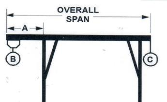
PROPER CANTILEVER PROCEDURES Required counterweight should not be supported by gantry caster frame.
